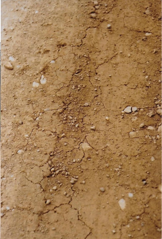
Photos of Farmington Township Roads. Note the color, lack of gravel, sodic surface cracking appearance-- are all tell-tale signs of excessive road spreading of oil and gas drilling wastewater.
